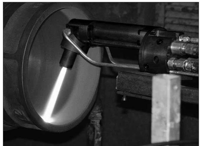
Fig. 18 Internal coating of a liner of a lokomotive diesel engine with ID CoolFlow
