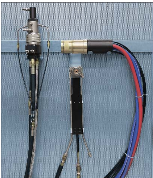
The jam box allows a parallel connection of the CJS, A60 and Axial III torches, for example.
